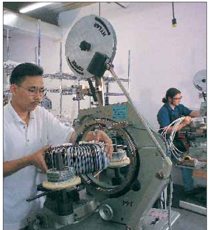
Applying Part of the Insulation System
