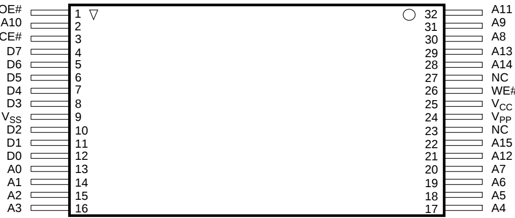
32-Pin — Standard Pinout
