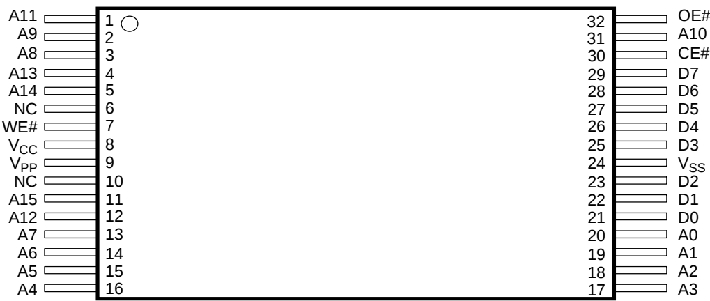
32-Pin — Standard Pinout
