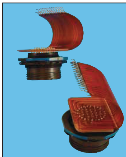
Flex Termination Assemblies
