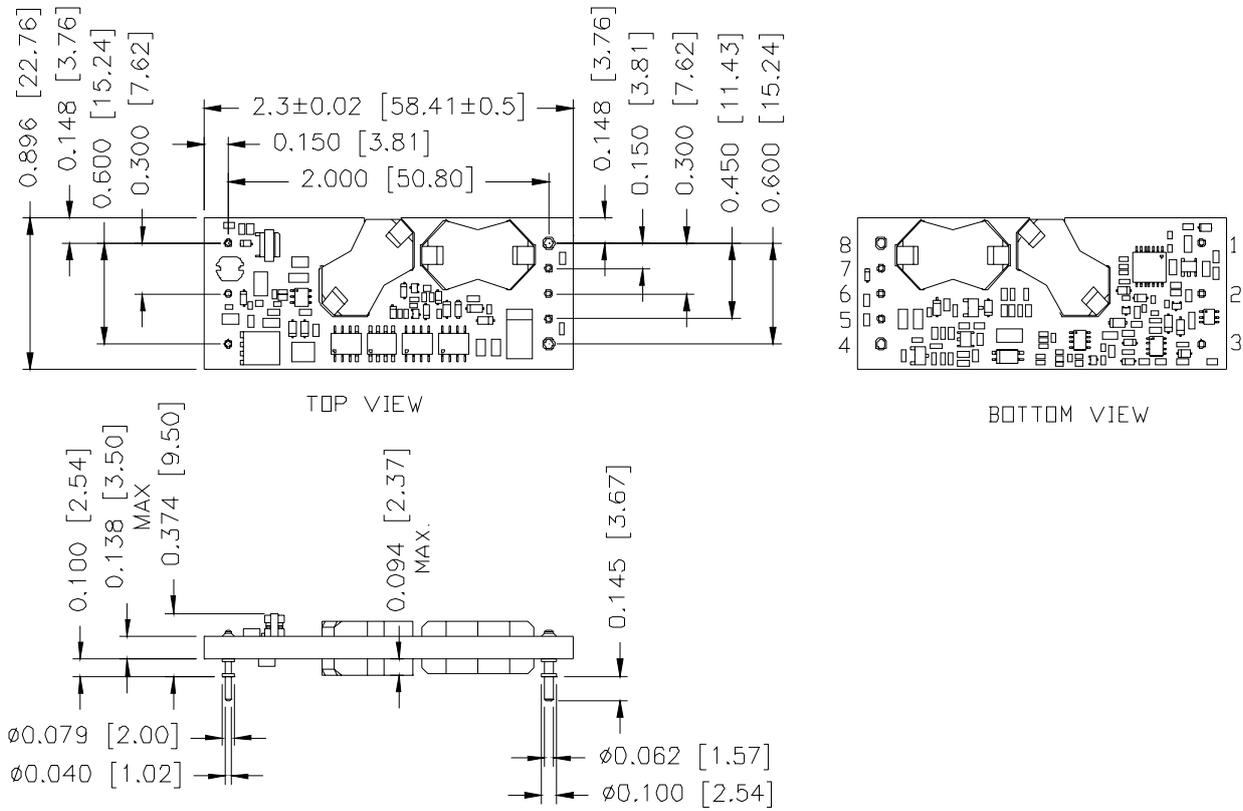
**Note:** The module doesn't guarantee at least 0.7mm as clearance distance on bottom side. This issue should be considered if any copper traces are on the top side of the user's board.
