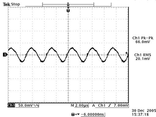
$V_{in} = 72\text{ V}$  and  $I_{out} = 15\text{ A}$
