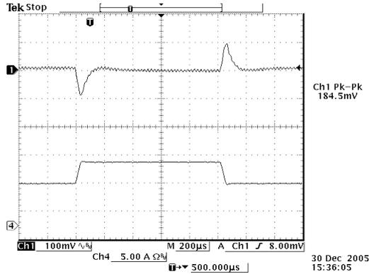
**Note:** Dynamic load transient at  $V_{in} = 48\text{ V}$ ,  $T_a = 25\text{ }^\circ\text{C}$ ,  $I_o = (50\% \sim 75\% \sim 50\%) I_{onom}$ ,  $di/dt = 0.1\text{ A}/\mu\text{S}$ .
