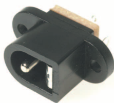
DC-13 panel mounting pin / ring type with switch. Rated 12V / 5A. DC-13A with 2.1mm dia. pin. DC-13B with 2.5mm dia. pin. DC-13A (FC681492) DC-13B (FC681493)
