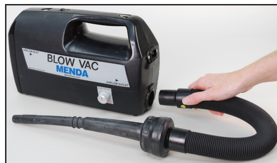
Figure 2: Connecting the hose to the airflow outlet.
