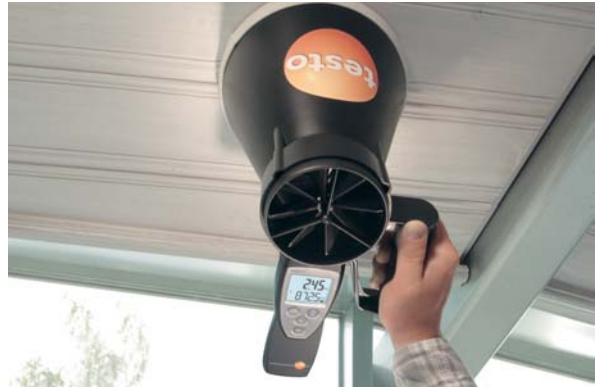
Using the testo 417 to monitor the air input at a ventilation outlet
