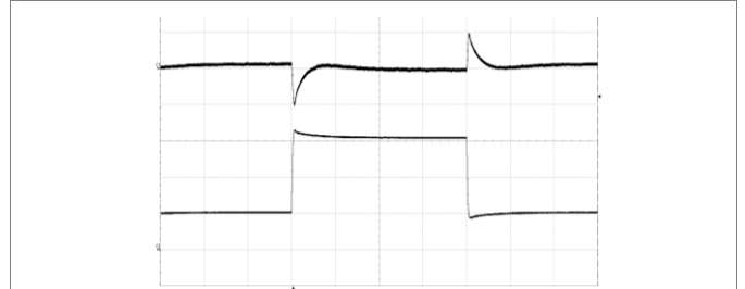
Output disabled by removing V_i at: T_{P1} = +25^\circ\text{C} , V_i = 48\text{ V} , I_o = 4.5\text{ A} electronic load. Top trace: output voltage (2 V/div.). Bottom trace: input voltage (20 V/div.). Time scale: (1 ms/div.).
