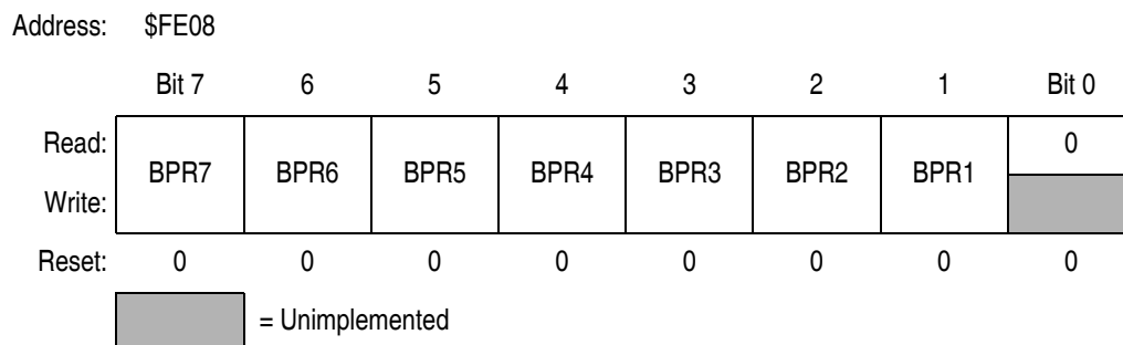
Figure 4-3. FLASH Block Protect Register (FLBPR)
