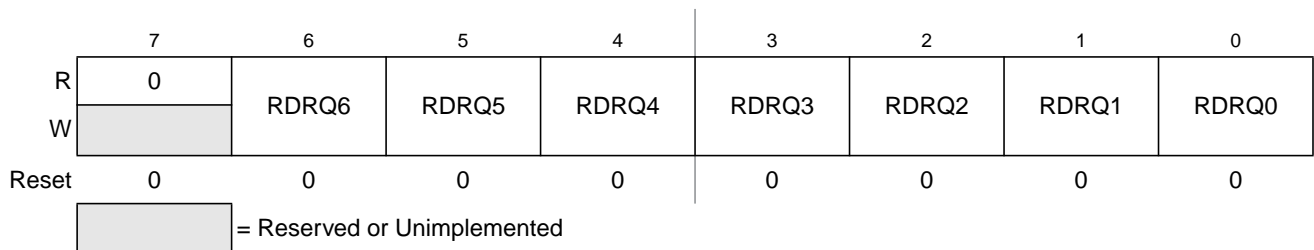
Figure 3-26. Port Q Reduced Drive Register (RDRQ)
