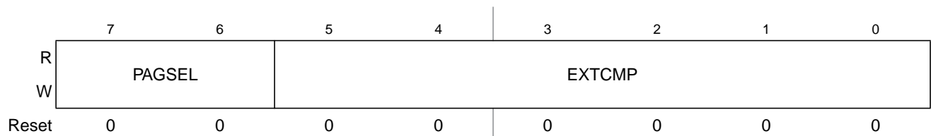
Figure 16-19. Debug Comparator B Extended Register (DBGCBX)
