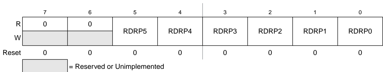
Figure 3-20. Port P Reduced Drive Register (RDRP)
