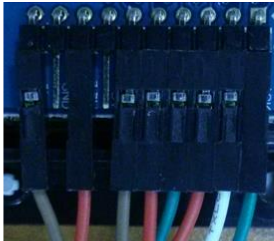
Figure 6-11 : Populated pins on FTDI Basic board.
