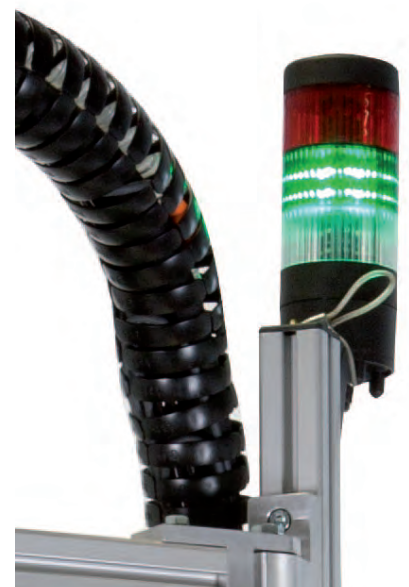
Signal lamps indicate the operating status
