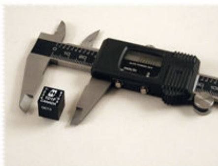
Caliper in photo opened to 1" (25.4mm)
