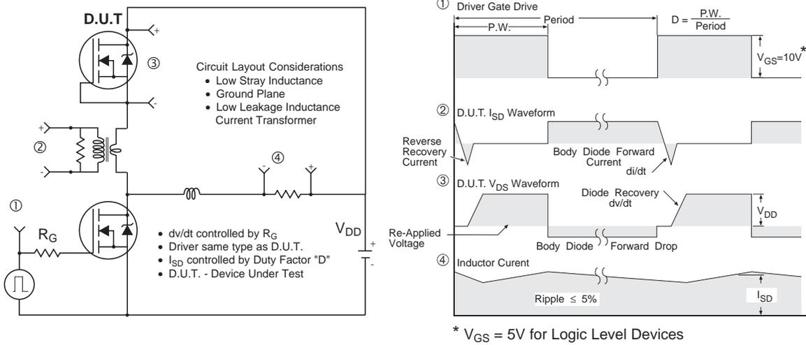
**Fig 15. Peak Diode Recovery  $dv/dt$  Test Circuit for N-Channel HEXFET<sup>®</sup> Power MOSFETs**
