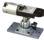
Crimp tool and Bench mount
