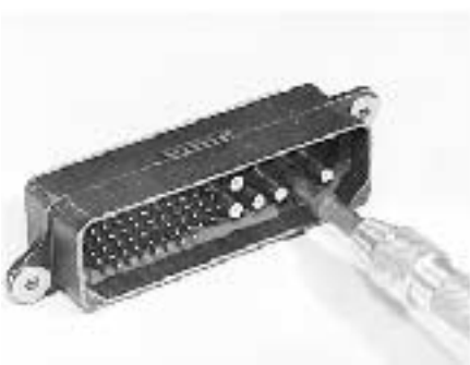
Extracting Coaxial & #12 Contacts
