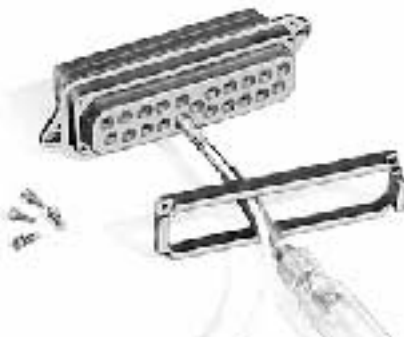
Inserting Coaxial & #12 Contacts
