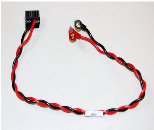
Figure 3: Power supply to driver board cable
