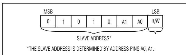
Figure 1. DS3502 Slave Address Byte
