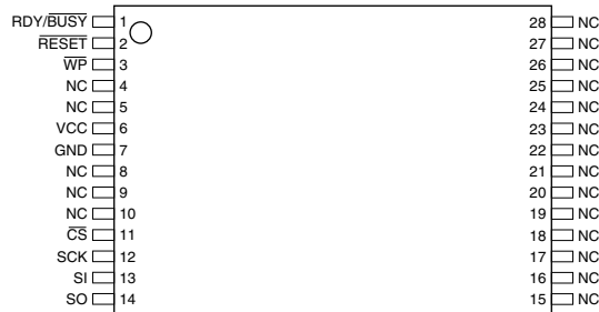
TSOP Top View – Type 1
