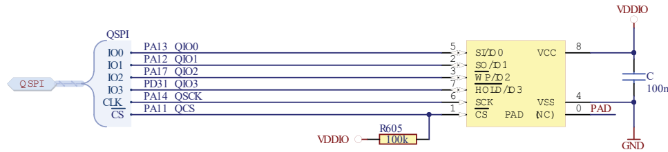
Figure 60-6. Schematic Example with QSPI Data Flash
