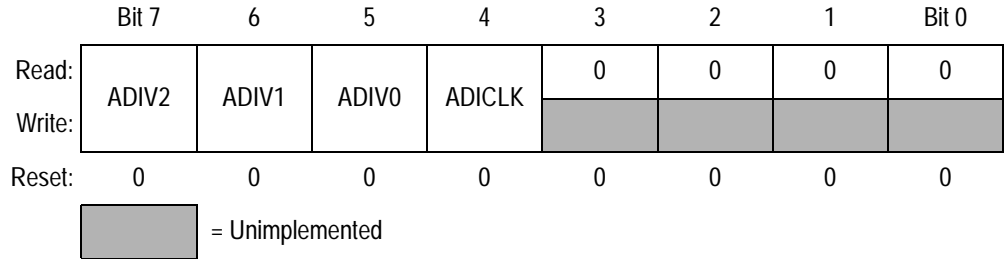
Figure 5-4. ADC Clock Register (ADCLK)
