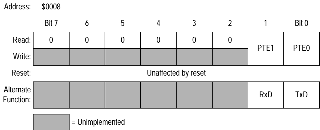
Figure 16-17. Port E Data Register (PTE)
