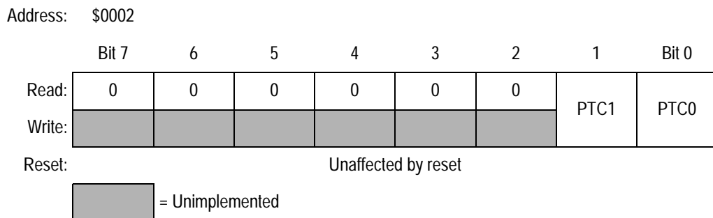
Figure 16-9. Port C Data Register (PTC)
