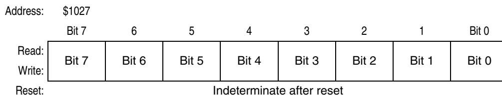
Figure 9-26. Pulse Accumulator Count Register (PACNT)
