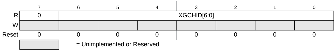
Figure 5-4. XGATE Channel ID Register (XGCHID)
