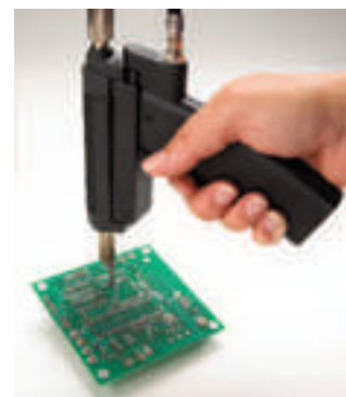
Through hole desoldering with the MX-DS1 hand-piece.
