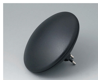
B5011129 ART-CASE R110 H PC+ABS (UL 94 V-0) black RAL 9005 ø4.33"x1.50" IP 40
