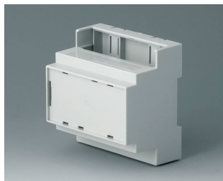
B6704107 RAILTEC C, 5 modules, Vers. IV PC (UL 94 V-0) light gray 3.46"x3.54"x2.28"
