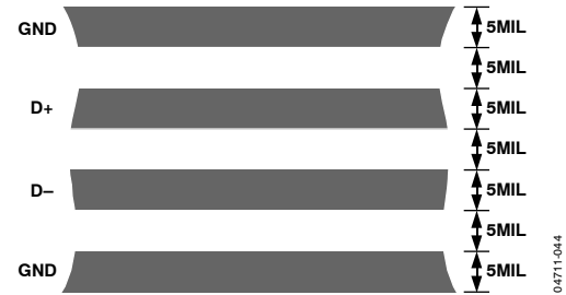
Figure 25. Arrangement of Signal Tracks
