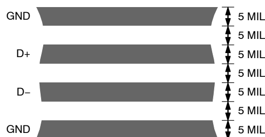
Figure 16. Arrangement of Signal Tracks
