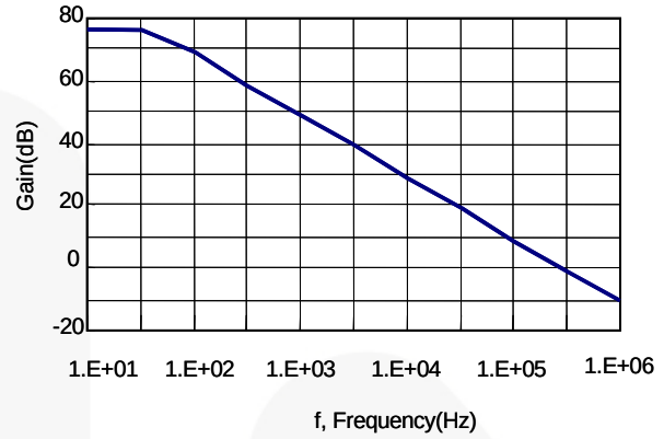
Figure 3. Open-Loop Voltage Gain
