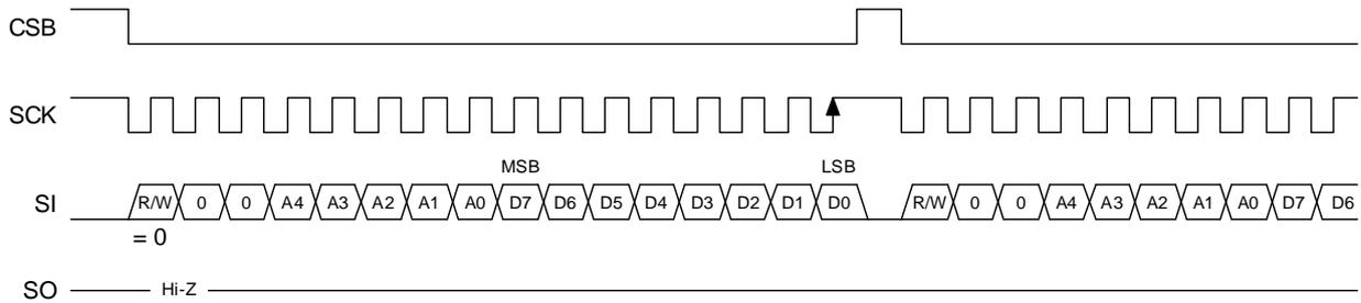
Figure 14.4 Random Address Access Mode Input Timing Diagram
