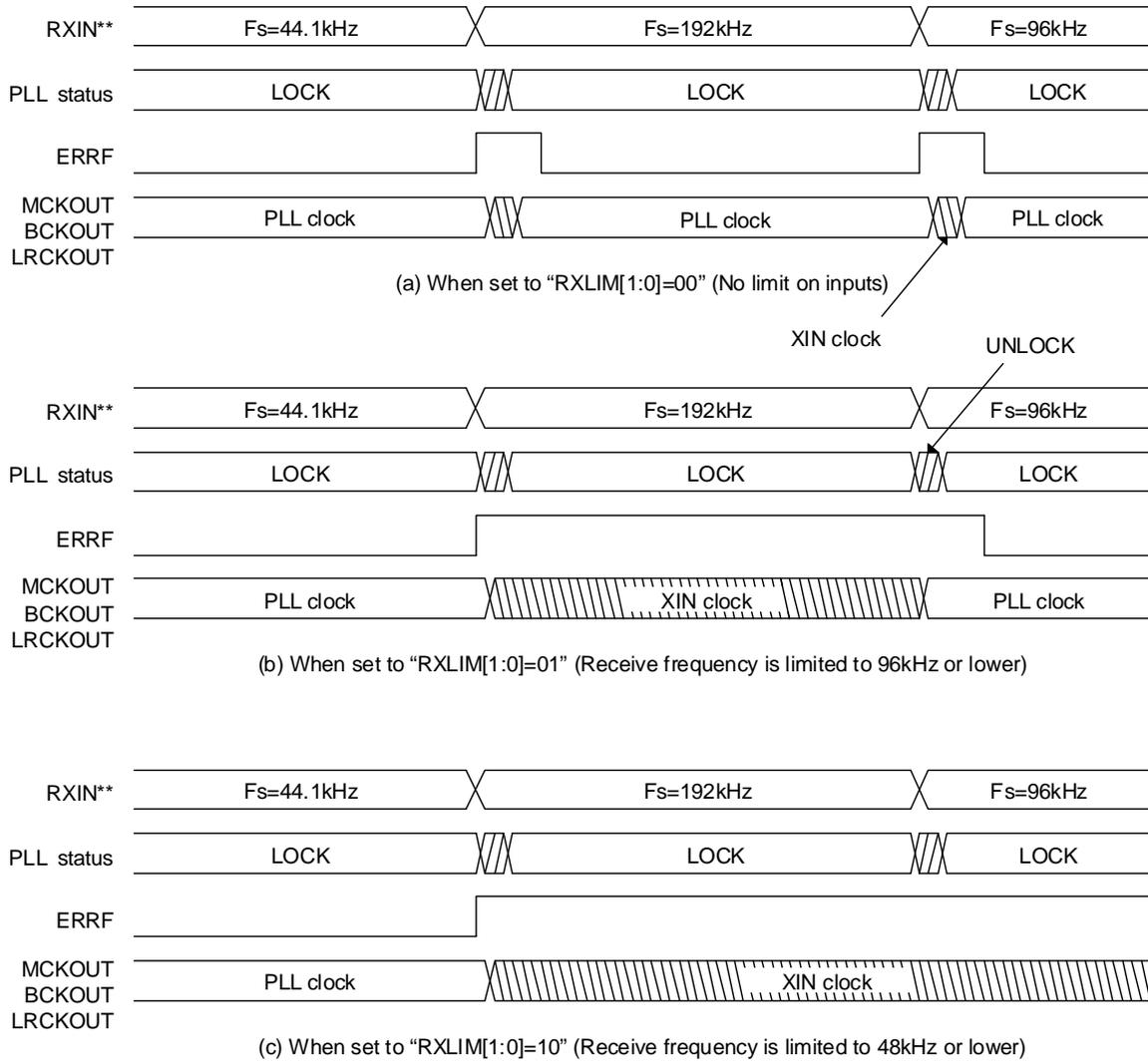
Figure 10.4 Output Clocks Generated When Input Data Reception Is Limited
