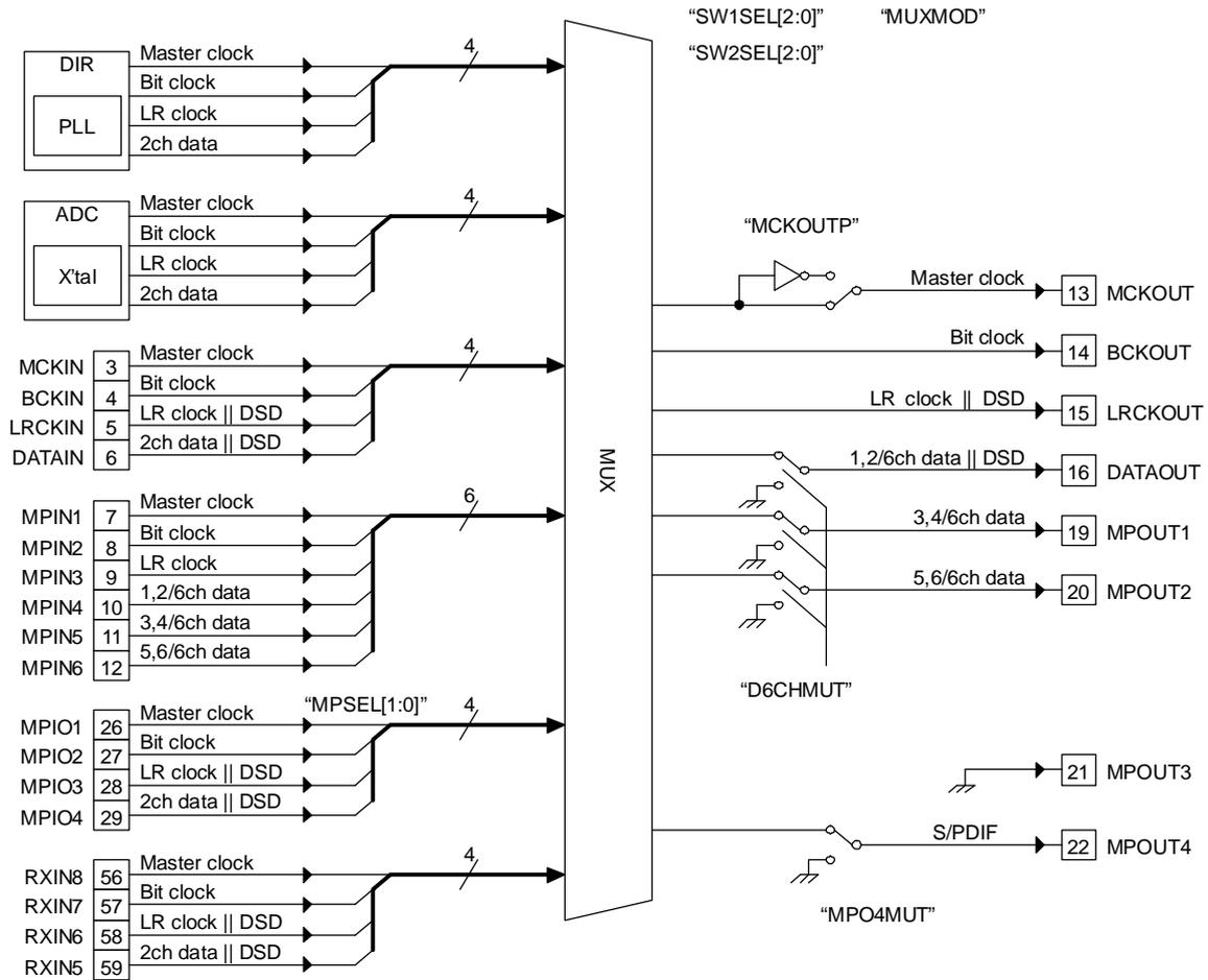
Figure 11.2 6-channel Data and 2-channel Data Support Audio Selector Configuration
