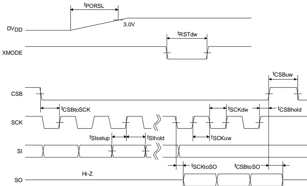
Figure 7.3 SPI Microcontroller Interface AC Characteristics
