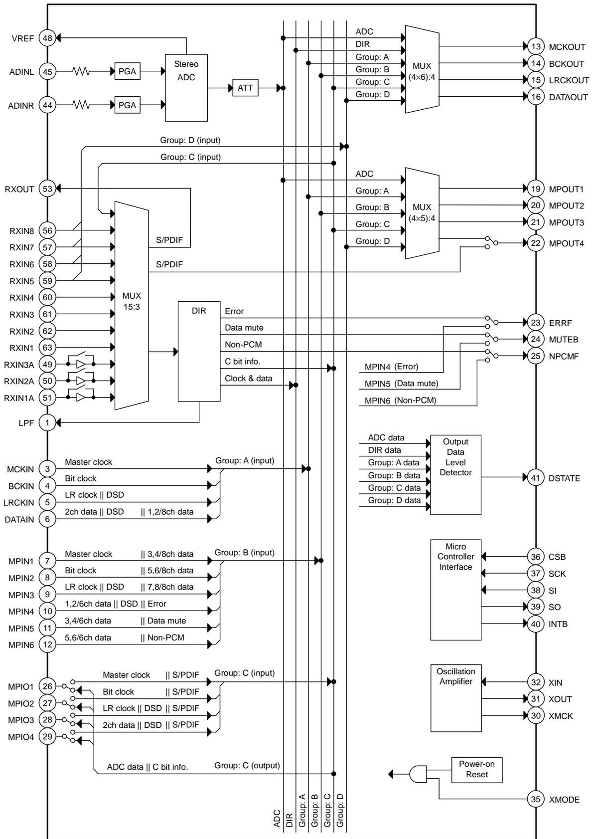
Figure 6.1 LC89075W-H Block Diagram
