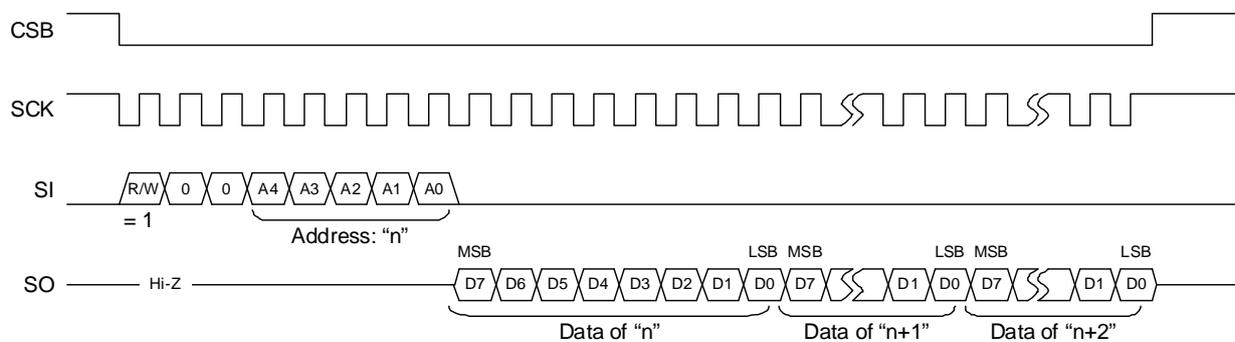
Figure 14.3 Current Address Access Mode Output Timing Chart
