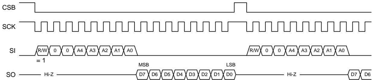
Figure 14.5 Random Address Access Mode Output Timing Diagram
