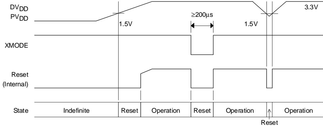
Figure 8.4 Power-on Reset and XMODE Reset Timing Chart
