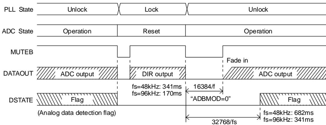
Figure 9.5 ADC Reset Processing Timing (When “ADBMOD=0”)
