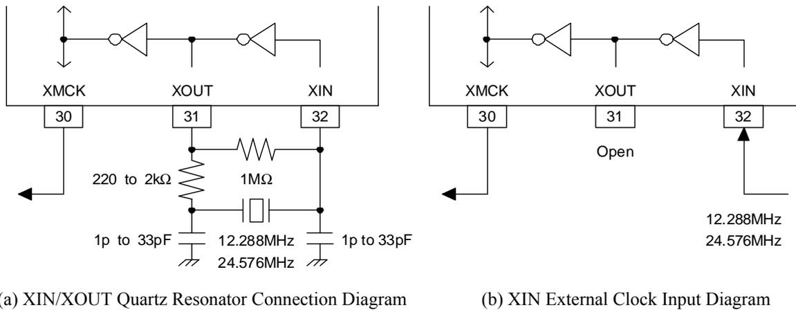
Figure 8.1 XIN/XOUT External Circuit Connection Diagram
