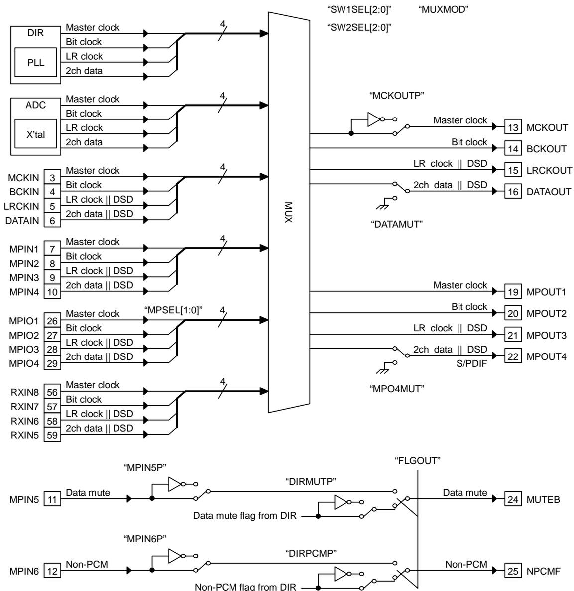
Figure 11.1 2-channel Data Support Audio Selector Configuration
