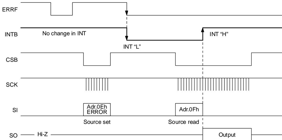
Figure 14.6 INTB Output Timing Example (when “INTBP=0”)
