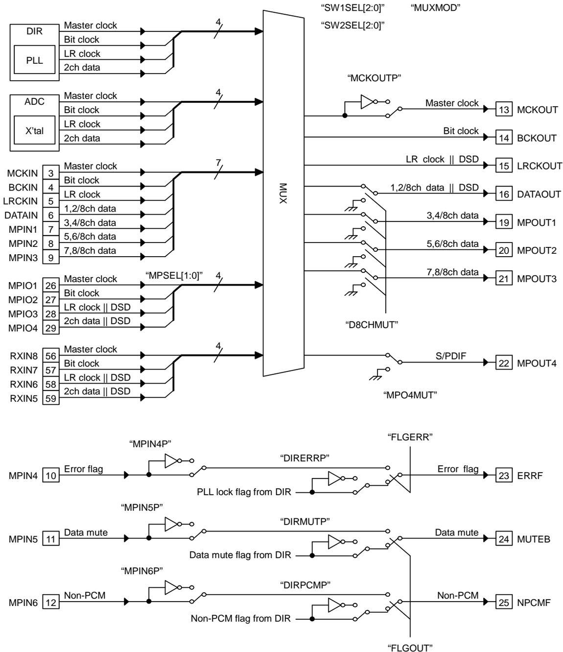
Figure 11.3 8-channel Data and 2-channel Data Support Audio Selector Configuration
