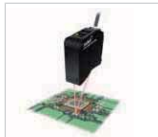
Measurement of the heights of chip parts
