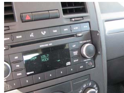
Bottom part in place without Nav
