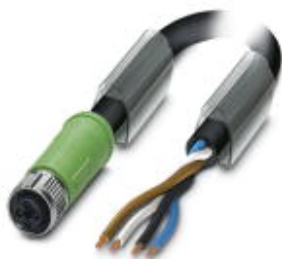
Power cable, 4-position, PUR halogen-free, black-gray RAL 7021, free cable end, on Socket straight M12 SPEEDCON, T-coded, cable length: 10 m
