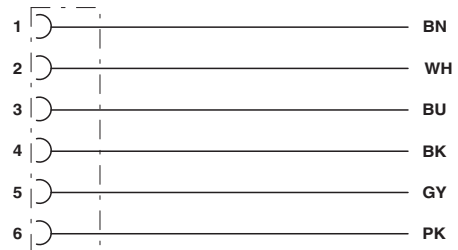
Contact assignment of M8 socket
