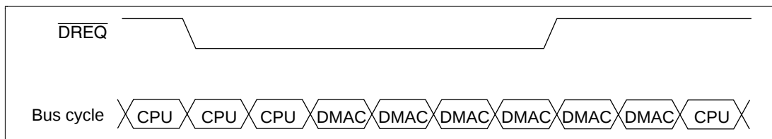
Figure 11.13 DMA Transfer Example in the Burst Mode
