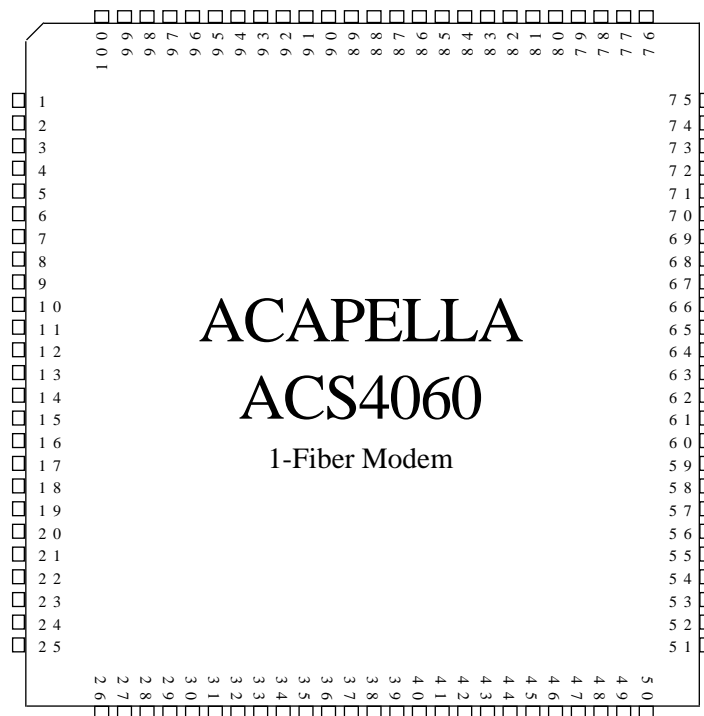
Figure 7. Top view of 100 pin TQFP package
