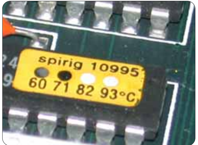
MICRO-CelsiStrip® with temperature levels 60 and 71°C surely exceeded. The 82°C never reached in the label's watch mission.
