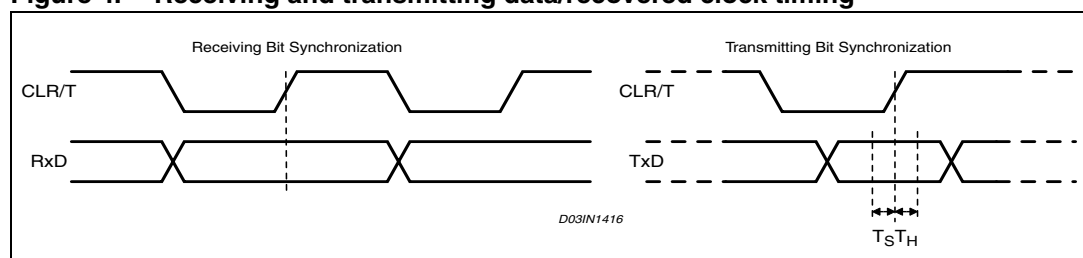
Figure 4. Receiving and transmitting data/recovered clock timing
