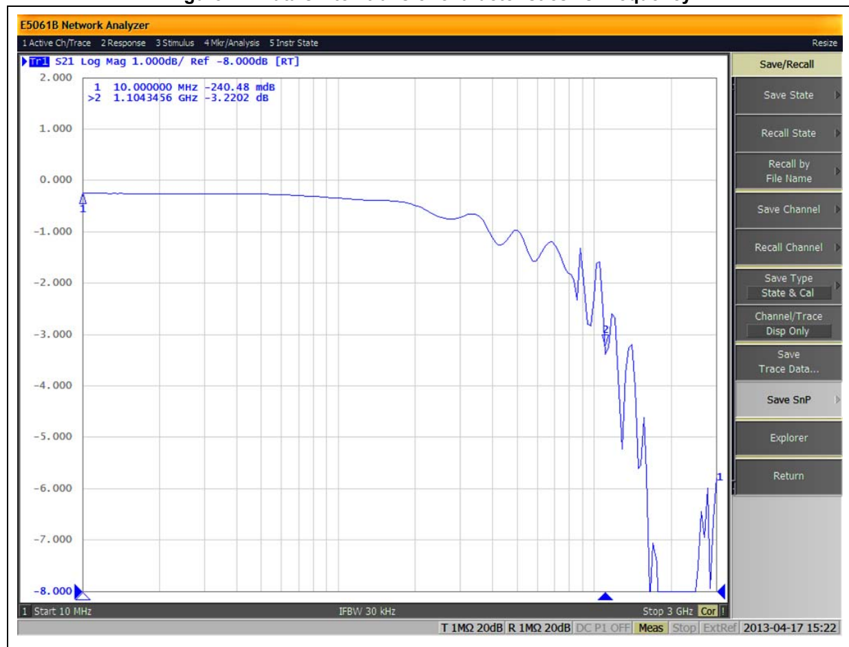
Figure 17. Data switch transfer characteristics vs. frequency
