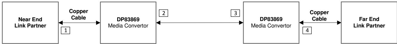
Figure 7-12. Link Loss Pass-Through
