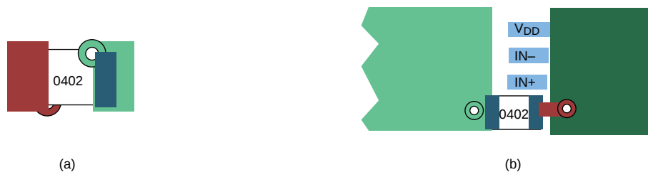
Figure 27. Typical Decoupling Capacitor Layouts
