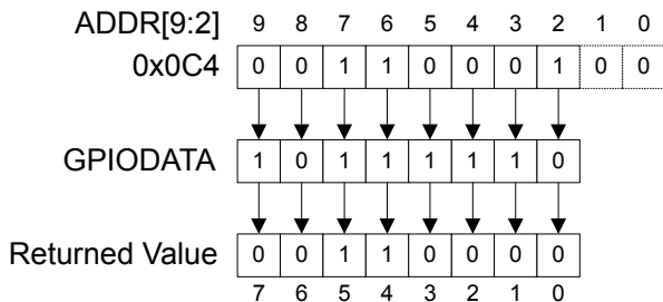
Figure 7-3. GPIODATA Read Example
