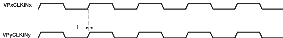
Figure 6-31. Video Port Dual-Display Sync Timing
