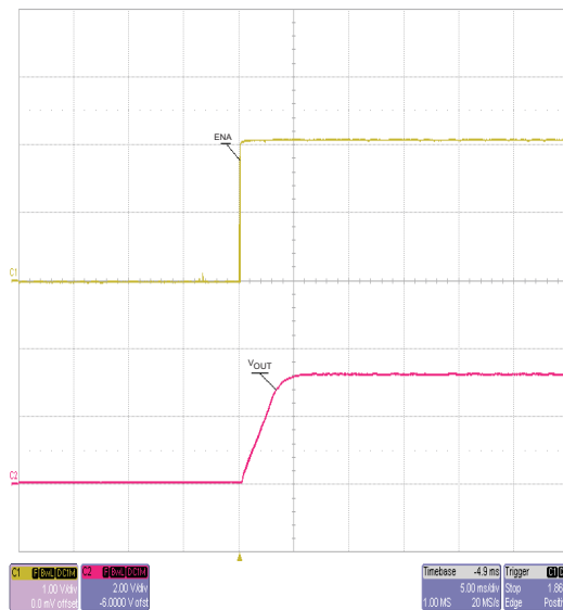
Figure 23. TPS54233 Start-up Relative to Enable
