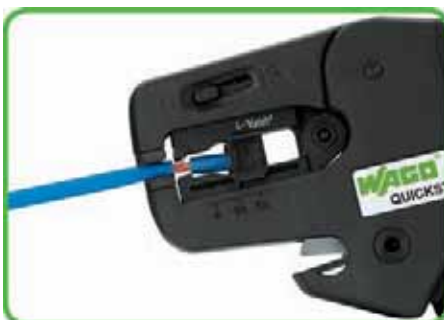
Stripping the conductor.
