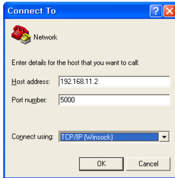
Figure 18. Network Terminal Program configuration
